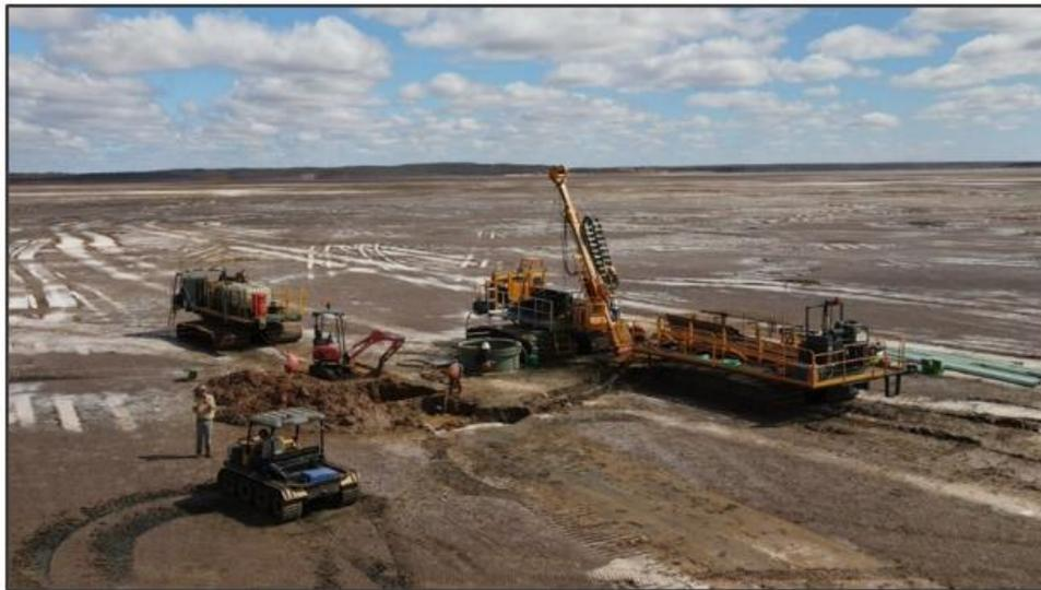
Figure 1: Raglan Drilling's lake rig sets up on first Sir Laurence diamond core hole
